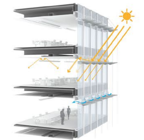
南立面遮阳措施 SHADING STRATEGY ON SOUTH FACADE
